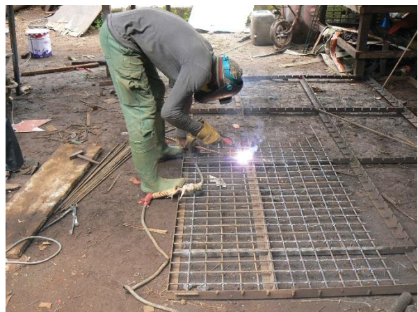
Image 21. Crafting of the rod mesh to build the platform for the Chimps in the Mainland.
