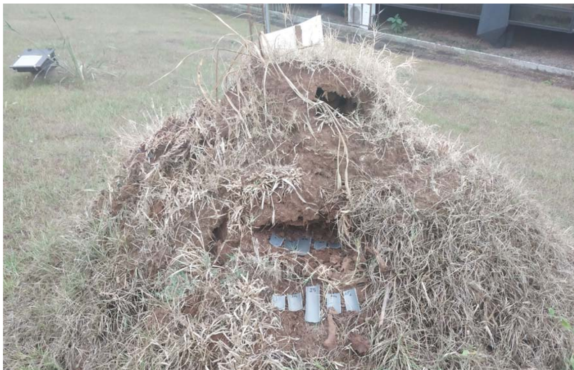
Termite proof? Test pieces of biocomposites using wood waste were placed on a termite mound to test their biodegradability. Photo: J.B. Saha Tchinda
