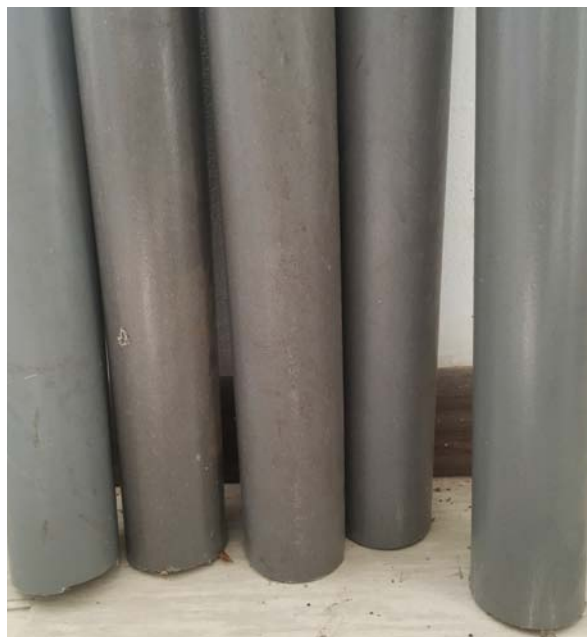
Pipe dream: The test products produced by mixing sawdust and PVC. Photo: J.B. Saha Tchinda
